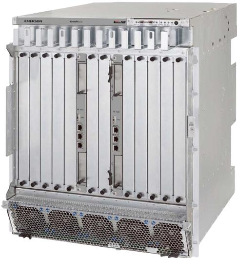
Centellis is architected to be a high availability platform suited to application acceleration and advanced networking with a rich ecosystem of blades and software that enable it to be deployed in a range of applications from security appliances to session border controllers to content optimization. Many configurations have been pre-certified for NEBS Level 3 saving both certification cost and time-to-market.
